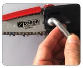
Tighten nut to fix bar cover
