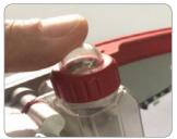
Oil tank for chain lubrication
